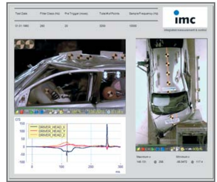
Synchronized playback of multiple videos, linked to time based data channel displays
